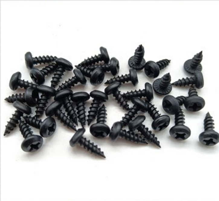
NAME: OVAL ROUND SELF TAPPING SCREW DIA: M3.5(#6)/ M3.9(#7)/ M4.2(#8) LENGTH: From 9mm to 30mm FINISH: Black/Grey Phosphated MATERIAL: C1022A
