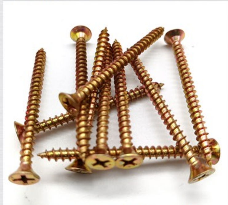
NAME: FINE THREAD BUGEL HEAD DRYWALL SCREW DIA: M3.5(#6)/ M3.9(#7)/ M4.2(#8)/ M4.8(#10) LENGTH: From 13mm(1/2") to 254mm(10") FINISH: White/Yellow Zinc Plated MATERIAL: C1022A
