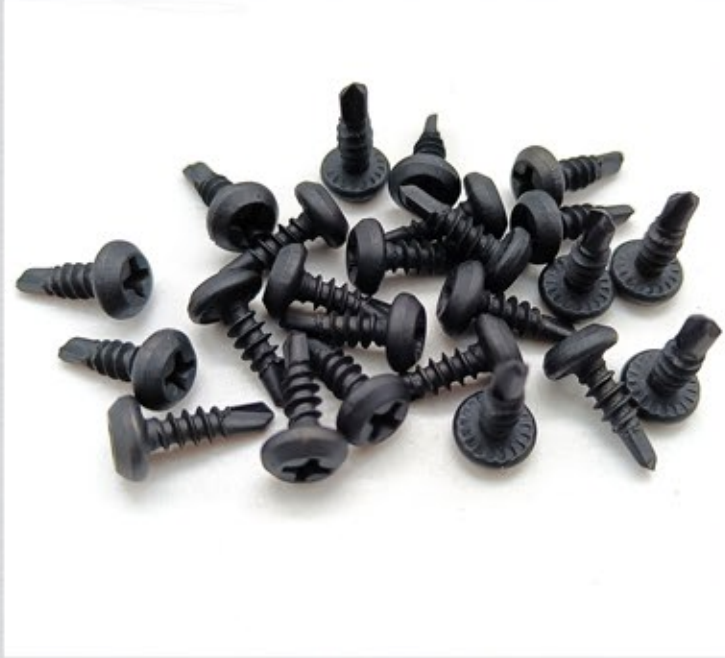
NAME: PAN FRAMING SELF DRILLING SCREW DIA: M3.5(#6)/ M3.9(#7) LENGTH: From 9.5mm to 13mm FINISH: Black/Grey Phosphated MATERIAL: C1022A
