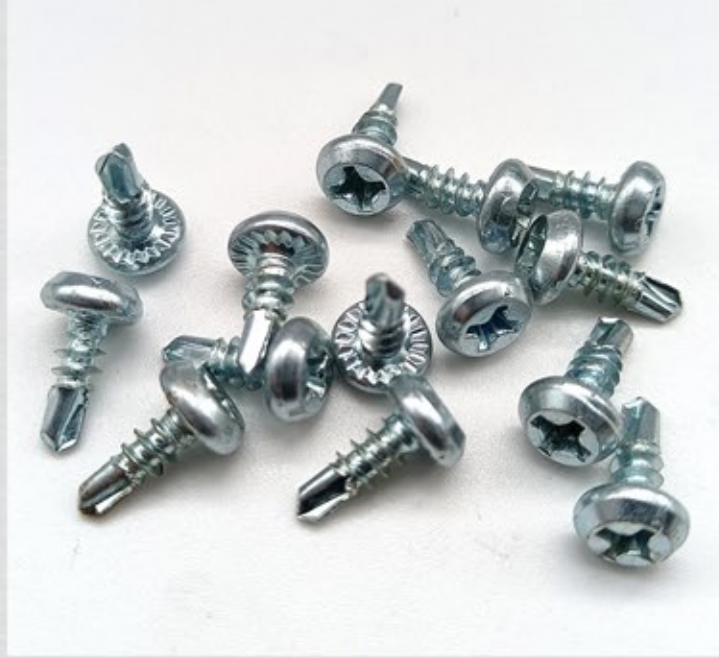
NAME: PAN FRAMING SELF DRILLING SCREW DIA: M3.5(#6)/ M3.9(#7) LENGTH: From 9.5mm to 13mm FINISH: White/Yellow Zinc Plated MATERIAL: C1022A
