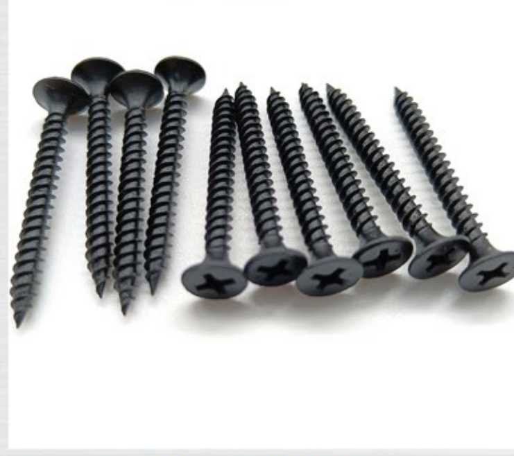
NAME: FINE THREAD BUGEL HEAD DRYWALL SCREW DIA: M3.5(#6)/ M3.9(#7)/ M4.2(#8)/ M4.8(#10) LENGTH: From 13mm(1/2") to 254mm(10") FINISH: Black/Grey Phosphated MATERIAL: C1022A
