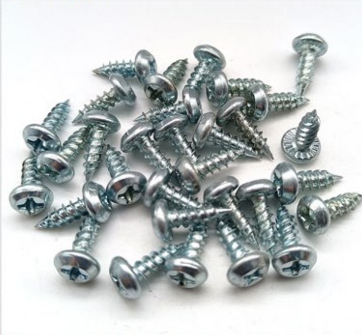
NAME: OVAL ROUND SELF TAPPING SCREW DIA: M3.5(#6)/ M3.9(#7)/ M4.2(#8) LENGTH: From 9mm to 30mm FINISH: White/Yellow Zinc Plated MATERIAL: C1022A
