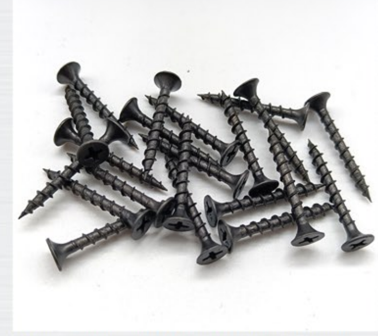
NAME: COARSE THREAD BUGEL HEAD DRYWALL SCREW DIA: M3.5(#6)/ M3.9(#7)/ M4.2(#8)/ M4.8(#10) LENGTH: From 13mm(1/2") to 254mm(10") FINISH: Black/Grey Phosphated MATERIAL: C1022A
